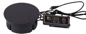
Induction Warmer 1AIW110V2 use as flush mount or with Domino stands (see page 16) only 2.61 amps 7 units per 20 amp circuit
